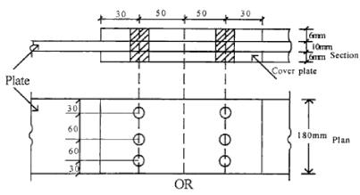
Determine the load carrying capacity of the joint as shown in figure. For 5mm weld. Assume field welding.
