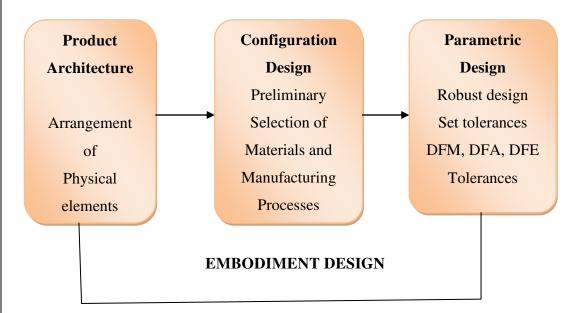
a) Product architecture: Product architecture is concerned with dividing the overall Design system into subsystems or modules. In this step we decide how the physical components of the design are to be arranged and combined to carry out the functional duties of the design.
