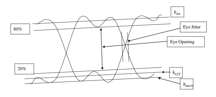
Fig.4.3 General Configuration of an eye diagram
