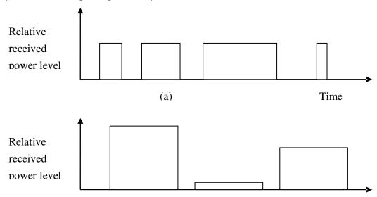
Fig.4.4 (a) Typical received data pattern in \_\_(b)\_\_ntional point to point links; (u) Optical signal level variations in pulses that may arrive at OLT
