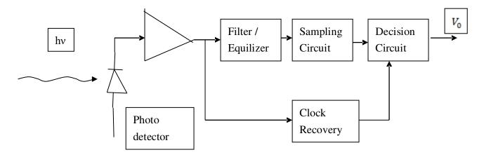
Fig. 4.2 The basic sections of an optical Receiver
