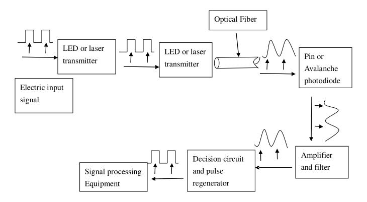
Fig. 4.1 Signal path through an optical data Link
