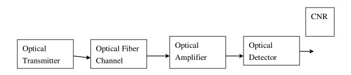
Fig. 4.4 Basic Elements of Analog Link
