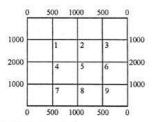
iterate by Gauss-Seidel method.
