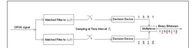
Receiver structure for QPSK. The matched filters can be replaced with correlators. Each detection device uses a reference threshold value to determine whether a 1 or 0 is detected.
