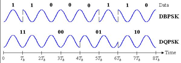
Timing diagram for DBPSK and DQPSK. The binary data stream is above the DBPSK signal. The individual bits of the DBPSK signal are grouped into pairs for the DQPSK signal, which only changes every  $T_s = 2T_b$ .
