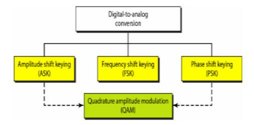
All convey data by changing some aspect of a base signal, the carrier wave (usually a sinusoid), in response to a data signal. In the case of PSK, the phase is changed to represent the data signal. There are two fundamental ways of utilizing the phase of a signal in this way:
