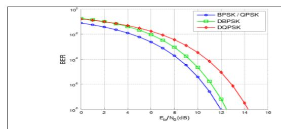
BER comparison between DBPSK, DQPSK and their non-differential forms using gray-coding and operating in white noise.
