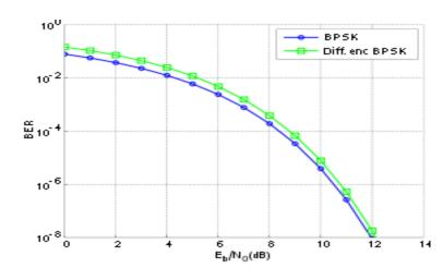
BER comparison between BPSK and differentially encoded BPSK with gray-coding operating in white noise.
