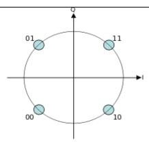
Constellation diagram for QPSK with Gray coding. Each adjacent symbol only differs by one bit.
