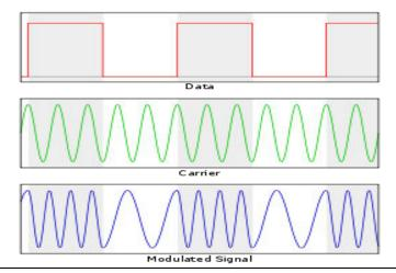
Frequency modulation in general changes the center frequency over time:
