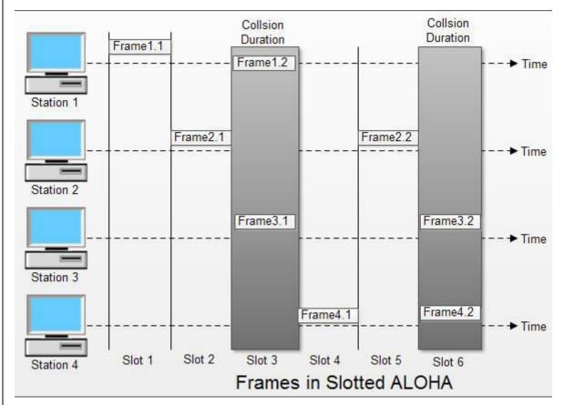
In slotted ALOHA, if any station is not able to place the frame onto the channel at the beginning of the slot *i.e.* it misses the time slot then the station has to wait until the beginning of the next time slot.
