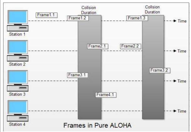
In fig there are four stations that .contended with one another for access to shared channel. All these stations are transmitting frames. Some of these frames collide because multiple frames are in contention for the shared channel. Only two frames, frame 1.1 and frame 2.2 survive. All other frames are destroyed.
