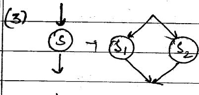
$$\text{gen}[s] = \text{gen}[s_1] \cup \text{gen}[s_2]$$
