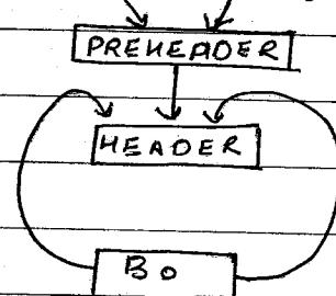
(4) Pre-Header - The pre-header is a new block created such that successor of this block is the header block. All the computations that can be made before the header block can be made before the pre-header block.
