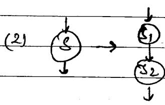
$$\text{gen}[s] = \text{gen}[s_2] \cup (\text{gen}[s_1] - \text{kill}[s_2])$$
