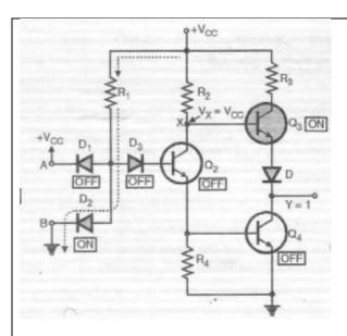
When AB = 11 then Vc is much more than 0.7 V and Transistor Q1, Q2 and Q4 is ON and Q3 is OOF and Y=0. Hence follows NAND operation.
