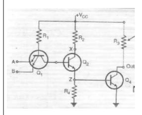
Equivalent circuit as shown for AB = 00, 01, 10, Y=1 and AB=11 (as shown) Y = 0. NAND operation.
