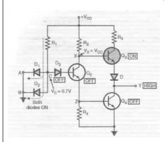
When AB = 01, 10 then Vc is at 0.7 V and Transistor Q1, Q2 and Q4 is OFF and Q3 is ON and Y=1.
