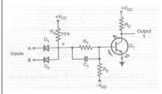
For AB = 00,01,10 the point x will be at 0.7V and equivalent diagram is as shown below
