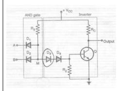
Fan out can be increased by replacing D3 with Transistor Q2.
