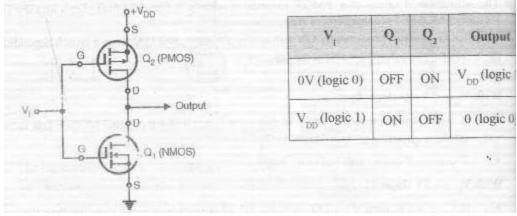
When Vi=0 then Q1=OFF,  $V_{GS}$  of Q2 = - $V_{DD}$  Q2=ON, hence Y=1 When Vi=1 then Q1=ON , Q2 = OFF hence Y=0
