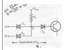
When AB = 00 then Vc is at 0.7 V and Transistor Q1, Q2 and Q4 is OFF and Q3 is ON and Y=1.
