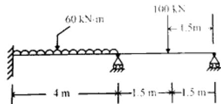
2. Analyse the continuous beam by stiffness matrix method. E is constant and relative I values are indicated on the beam. 14
